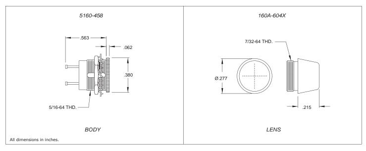
These Gemlite Indicator Lights are a versatile design capable of accepting all T-1 sub-midget flange based lamps. These high quality indicators provide reliable service in a vast array of military and commercial applications where a miniature relampable front panel indicator is required. The lamp is not included with this indicator light. Please order the required lamp separately.
